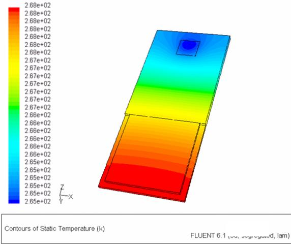
Fig. 1: Hot dissipater temperature distribution.
