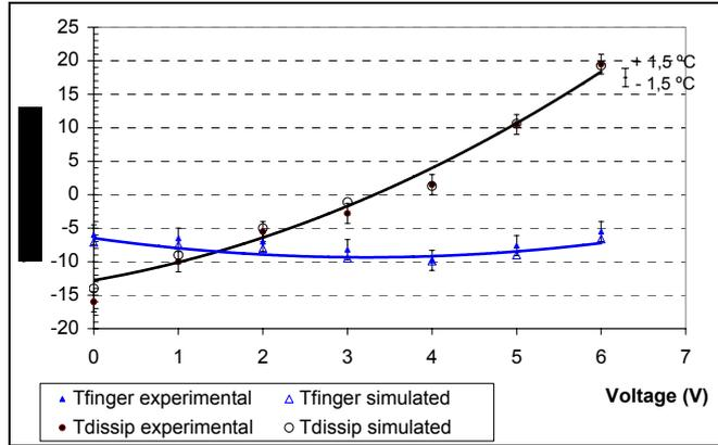
Fig. 5: Comparison of the simulated and the experimental temperatures of the ice maker.
